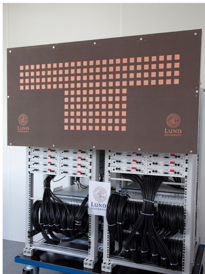
The massive MIMO testbed at Lund University in Sweden is based on USRP RIO with a custom cross-polarized patch antenna array.
