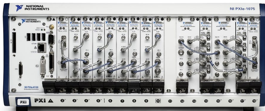
PXI Express modular vector signal analysers and generators, with LOs daisy-chained from module to module.
